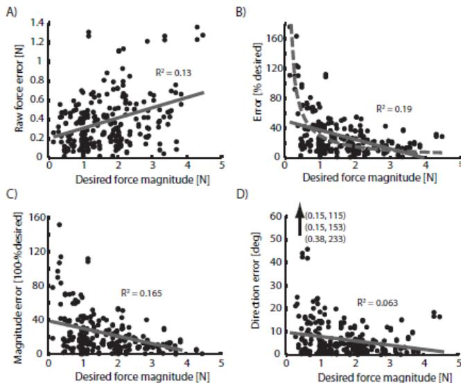
Fig. 8. Error metrics with respect to desired force magnitude. A) Raw force error. B) Normalized error. C) Magnitude error. D) Direction error. Each point corresponds to a single force trial. Five different experiments are represented. Linear fits and their corresponding  $R^2$  values were reported. An inverse relationship between normalized error and force magnitude was also shown in B) as a grey, dashed line.
