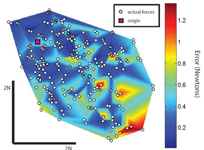
Fig. 7. Contour plot of the raw error during feedforward FES control of isometric forces. The error in regions unoccupied by actual forces (white circles) was interpolated.
