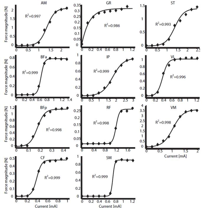
Fig. 4. Recruitment curves for the 11 muscles used for control. The individual points (black diamonds) correspond to the average steady-state force at the given current or stimulation strength. The sigmoid curves were fit to this force data and  $R^2$  values quantified the goodness of fit.
