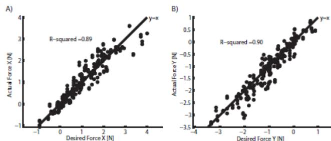
Fig. 6. Correlations between actual and desired force components. A) Forces in the x-direction. B) Forces in the y-direction. Data combined from five different experiments. Reported  $R^2$  is across all experiments.
