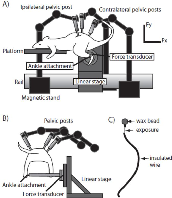
Fig. 1. Schematic of FES test platform. A) Illustration of pelvic fixation and ankle attachment to a force transducer. B) Rear view of test platform. C) Stimulation electrode design with an exposure that is situated near the motor point of targeted hindlimb muscles.
