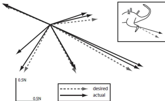
Fig. 5. Example force trials (black, solid vectors) of open loop FES control to desired force vectors (grey, dashed vectors) in the sagittal plane. Two repetitions to each desired force were performed non-sequentially. Refer to the inset for the relation between the forces and the rat hindlimb. Rat schematic modified from Tresch and Bizzi [29].
